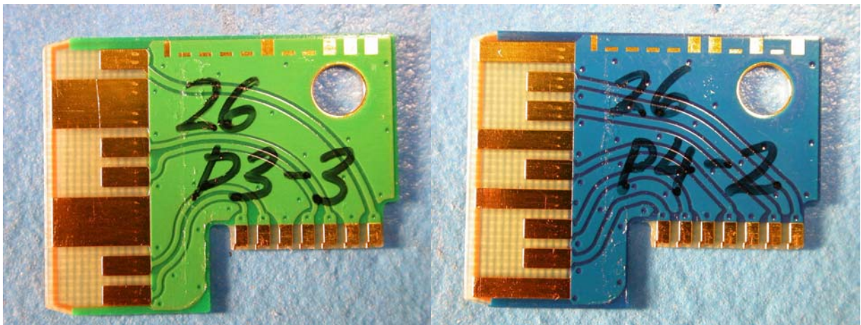
Fig. 15 Connector blades after vibration qualification
