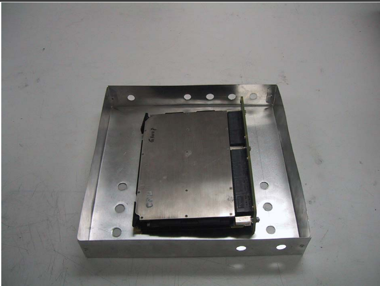
Fig. 38 Enclosure for salt + SO 2 test (top cover not shown)
