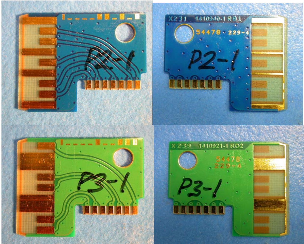
Fig. 41 Connector blades after 500 cycles of durability
