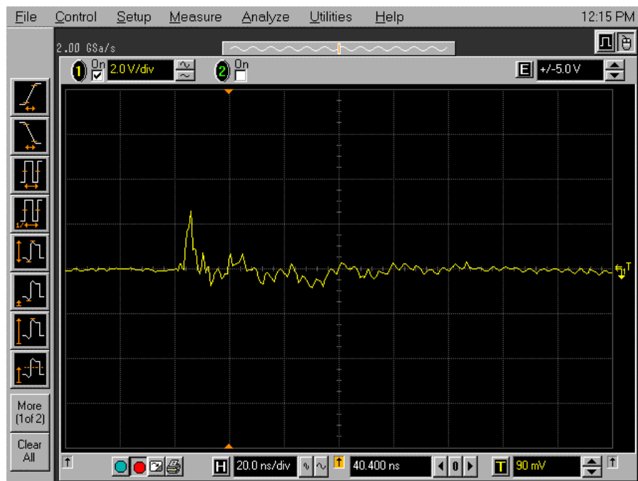
Fig. 49 Voltage response after 500 durability cycles (2.5 V peak)
